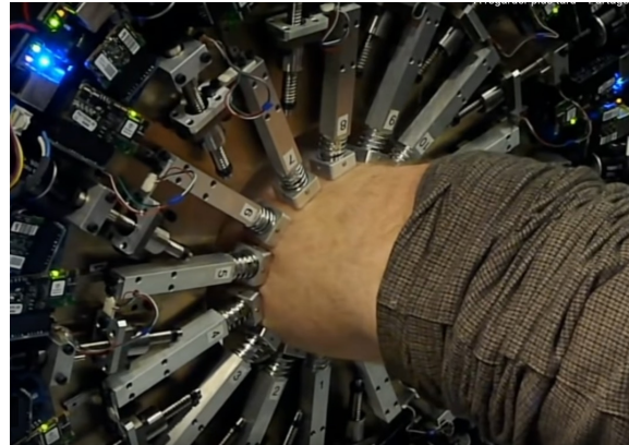
Customized robot to measure tissue characteristics
