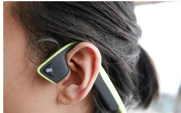
Earphone : transfers sound by bone vibration directly to the cochlea
